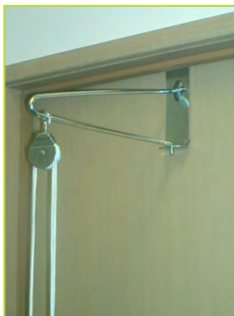
Assembled Pulley System Close up
